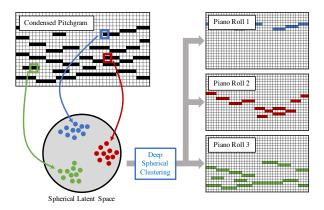
**Figure 1**. Each bin of a condensed pitchgram is embedded on a spherical latent space taking into account the timbral characteristics. Piano rolls of each instrument part is obtained by deep spherical clustering on the space.
