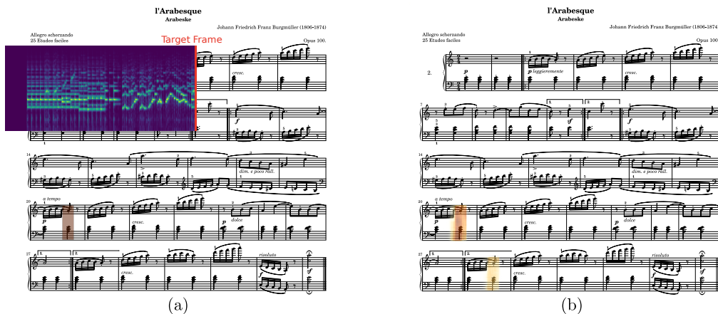
Figure 1. Score Following Task as modelled in this work: Given a score (sheet image) and an incoming musical performance (audio), the goal is to predict the current location in the score in real time. The audio is fed to the tracker frame by frame and the system processes the last 40 frames to predict the position for the latest frame (the Target Frame marked red in (a)). The ground truth (bounding box around current score position; see (a)) is given as a binary segmentation mask. The system predicts a probability for each pixel to correspond to the current audio; thus it highlights those regions that are most likely to match the correct location. Ideally, this should be only a single region. However, in (b) we see that such a prediction is not perfect: while the highest probability is assigned to the correct position in staff four, there is also a small likelihood in the last staff, as the notes are the same for both locations. To predict the location correctly, the system needs to consider the whole audio up to the current point in time, which motivates our design choices introduced in Section 3.
